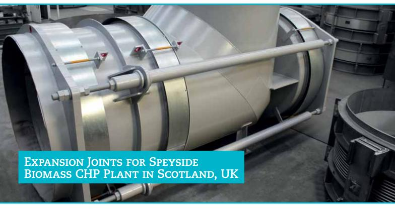
MACOGA supplied **Elbow Pressure** Balanced, Lateral and Hinged expansion joints DN2000 for Speyside Biomass CHP Plant in Scotland, UK.
