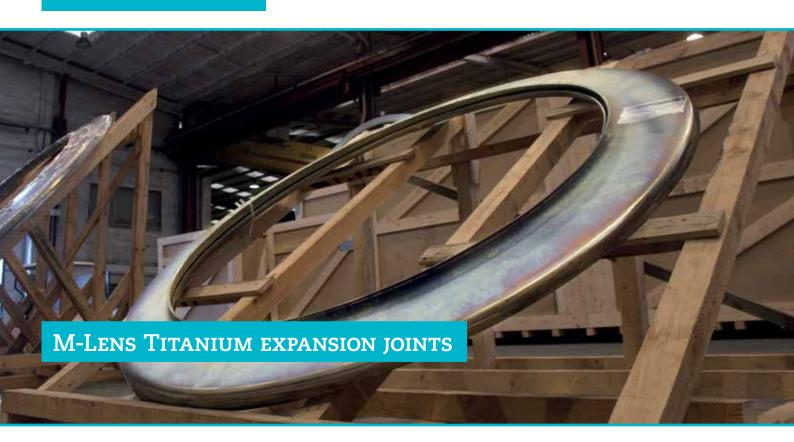
Two MACOGA **M-Lens expansion joints** in TITANIUM Gr. 2 (3.7035) have been successfully designed and manufactured at MACOGA.
